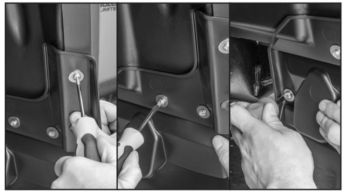
**12** While firmly pressing the MudFlap to the fender, fully tighten the top Phillips head screw with a Phillips screwdriver. Next, fully tighten the (2) hex head screws with a flat screwdriver. Then, using a stubby Phillips screwdriver, fully tighten the innermost Phillips head screw.
