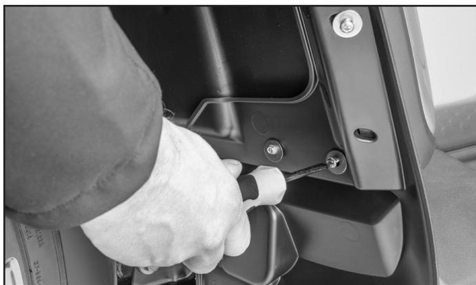
**10** Take (2) supplied flat washers and (2) supplied hex head screws and install them into the two holes in the MudFlap as shown with a flat screwdriver to a loose fit.
