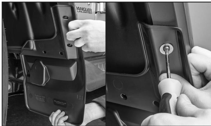
**8** Place the MudFlap marked, "LH," up to the fender and align with the corresponding holes. Then, take (1) supplied flat washer and (1) supplied coarse Phillips head screw and install into the top hole of the MudFlap to a loose fit with a Phillips screwdriver.
