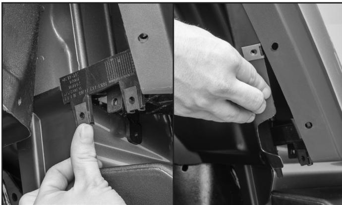
**7** With the inner fender pulled back, take (2) supplied wider u-clips and install over each factory hole as shown. Then, move the inner fender liner back into place.
