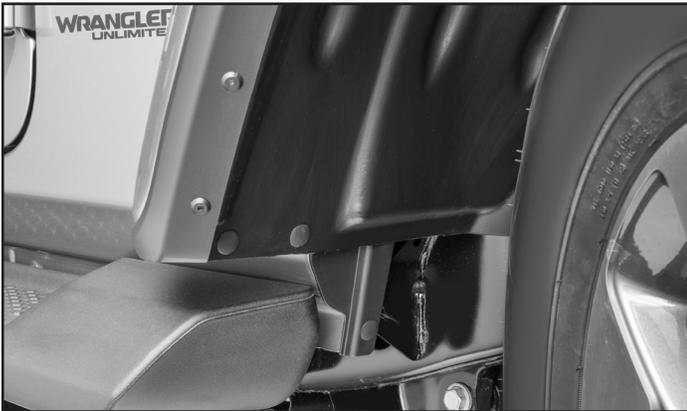
**13** Install the passenger side MudFlap marked "RH," with the wheels turned fully to the right repeating Steps 3-12.
