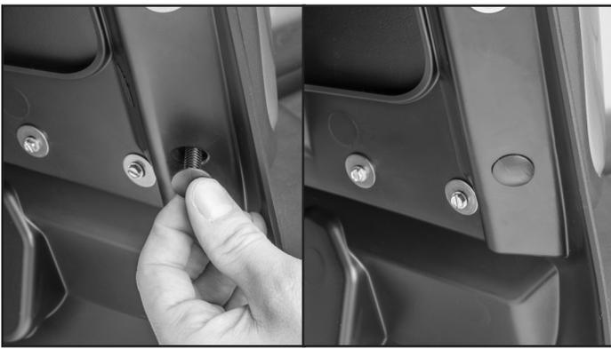
**11** Take (1) supplied plastic fastener and install into the remaining hole in the MudFlap.
