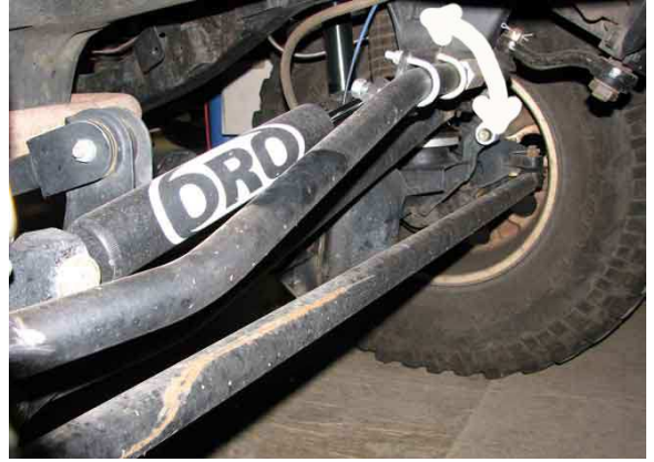
The picture on the right shows how you can rotate the draglink to ensure there is no contact to the tie rod, if there is, simply adjust the rotation of one tie rod end to prevent it from drooping that far.
