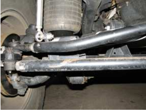
The picture on the left shows the point of contact area between the draglink and tie rod.
