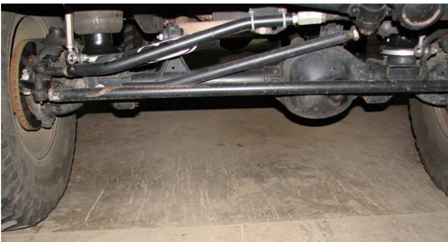
At ride height, with a long droop suspension, it is normal for the draglink to sit like shown in the image to the left.
