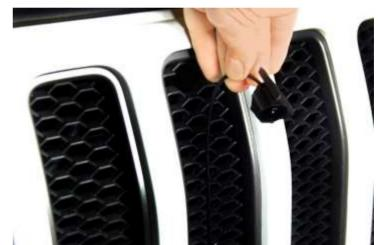
Start with removing the 5 clips holding the top of the grille to the core support. Once removed, you can lean the grill forward to aid in installation. Starting with the bottom tab, insert into grill then snap the upper camera mount into place. It is recommended to only lightly fit the mount into the grill and not snap it into place until the rest of the installation is complete to simplify aligning the camera.
