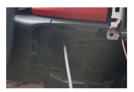
Using the wire routing diagram, run the camera wiring down the front of the vehicle and against the fender. The rear washer nozzle tubing hold down can be used to hold the camera wiring also. Run the wiring through the clutch plug and into the vehicle. Route under the dash and through the Push to start wiring hole. NOTE: It may be easier to first run the wiring through the firewall from inside the vehicle. Make sure to run wiring through clutch plug before running to the grill.
