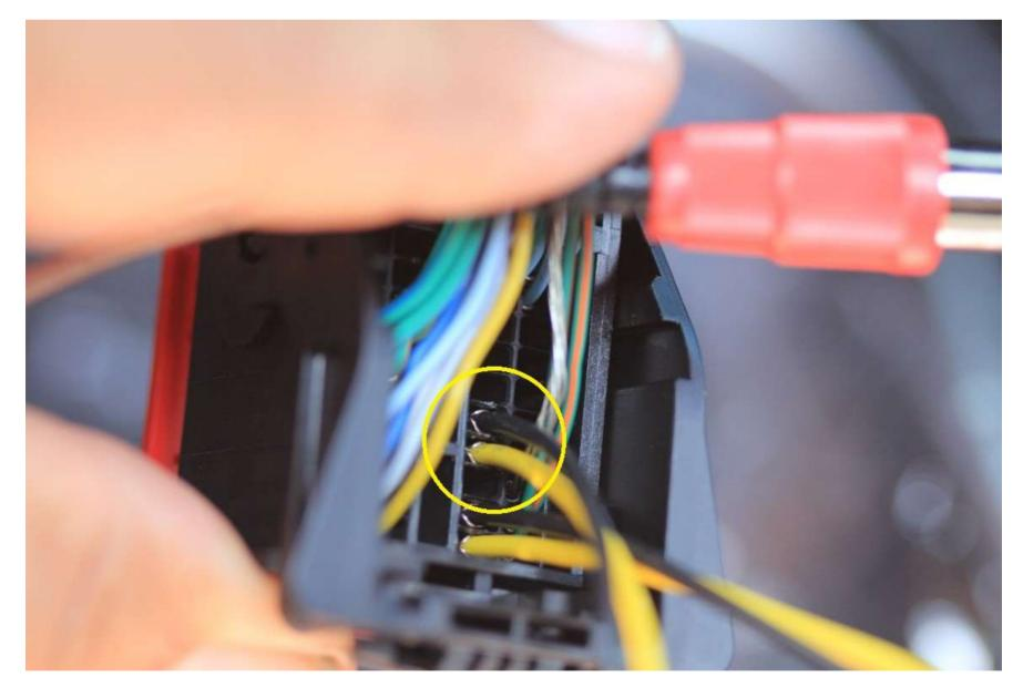
Using a small flat head screwdriver, remove the red terminal cover off the main radio connector. Once the cover is removed, plug the yellow wire into pin 24,and the black wire into pin 25. Once installed, reinstall the red terminal cover.
