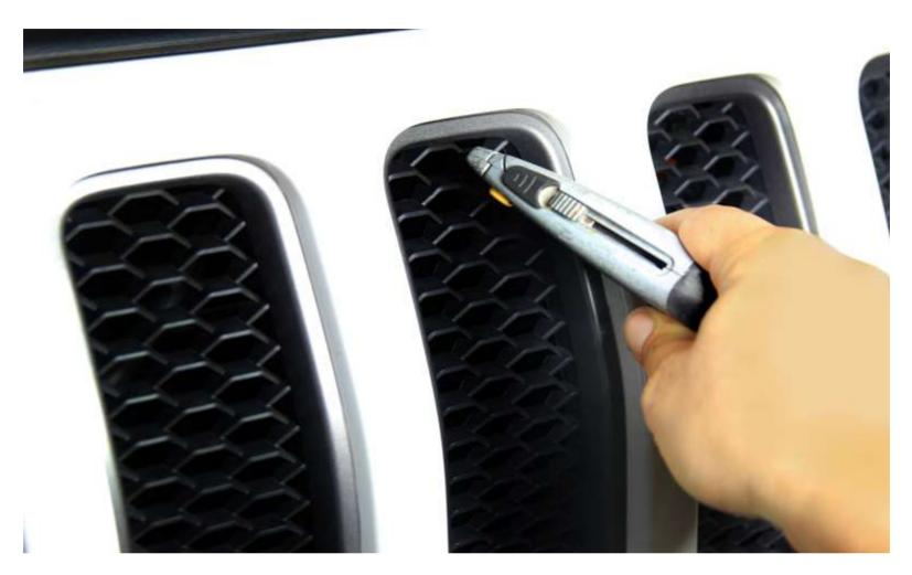
Using a box cutter or wire snips, trim middle grill slating to fit camera bracket
