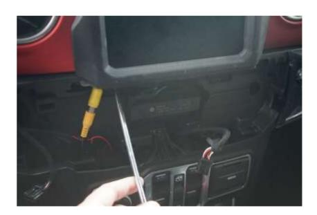
Using a Phillips head screwdriver, remove two screws holding radio bezel to dash. Once screws are removed, use a trim stick to remove bezel from dash.
