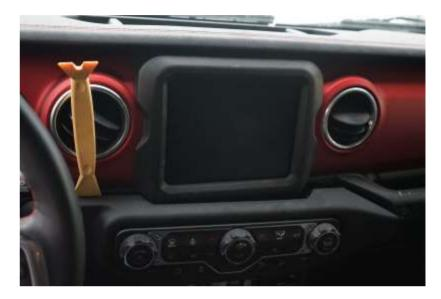
Step 2: Radio Bezel Removal
