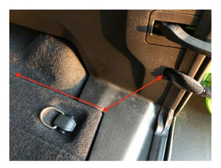
Removed the trail rails by popping off the plastic caps and removing the three bolt in a 2 Door. Ran the wire under the carpet to the right.
