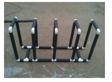
You then can go back and add the PVC cement to help stiffen and seal the frame. Final step is to mount the holder to the dolly with zip ties so you can roll it around. You can also add a couple of velcro straps to keep the doors together while rolling around the driveway.
