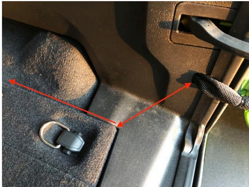
Removed the trail rails by popping off the plastic caps and removing the three bolt in a 2 Door. Ran the wire under the carpet to the right.
