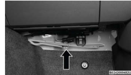
Auxiliary Switch Connections – Under Instrument Panel
