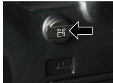
Rear Cargo Power Outlet
