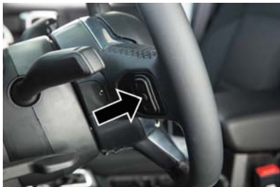
Audio Controls (Back View Of Steering Wheel)
