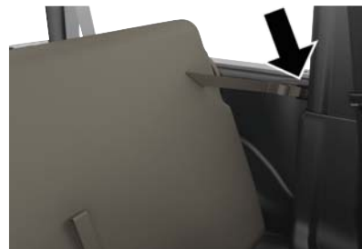
Rear Seat Tumble Position Retention Strap
