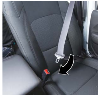
Inserting Latch Plate Into Buckle
