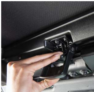
Squeeze Latch Plate And Pull Handle Upward
