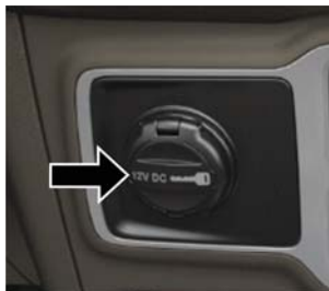
Front Power Outlet
