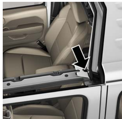
Torx Head Screw Location — Driver's Side Shown
