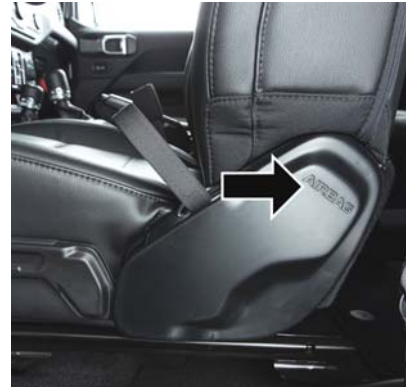
Supplemental Seat-Mounted Side Air Bag Location
