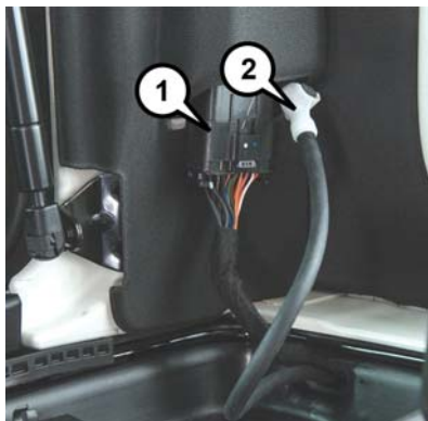
Wire Harness And Washer Hose Location
