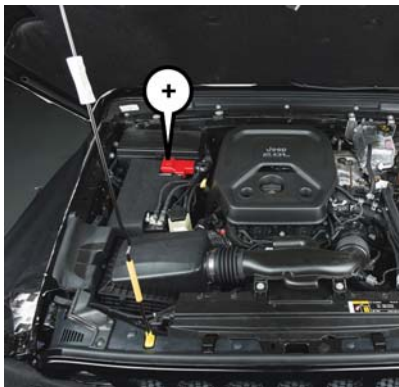
Positive Battery Post
