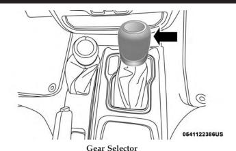
**NOTE:** If the gear selector cannot be moved to the PARK, REVERSE, or NEUTRAL position (when pushed forward), it is probably in the AutoStick (+/-) position (beside the DRIVE position). In AutoStick mode, the transmission gear (1, 2, 3, etc.) is displayed in the instrument cluster. Move the gear selector to the right (into the DRIVE [D] position) for access to PARK, REVERSE, and NEUTRAL.
