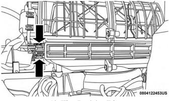
Air Filter Retaining Tabs
