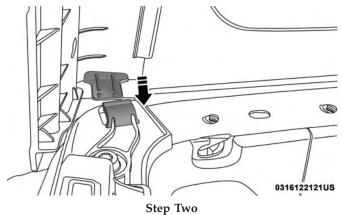
3. Engage the plastic retainers along the bottom of the quarter window and up the front of the window. Repeat on the other side.
