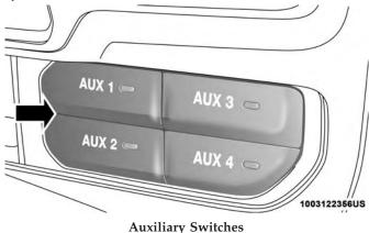
**NOTE:** Holding last state conditions are met when switch type is set to latching and power source is set to ignition.
