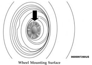
Tighten the lug nuts/bolts in a star pattern until each nut/bolt has been tightened twice. Ensure that the socket is fully engaged on the lug nut/bolt (do not insert it halfway).
