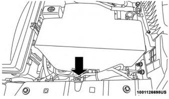
Auxiliary Switch Connections - Under Hood
