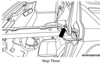
4. Remove the six Torx head screws that secure the hard top to the vehicle (along the interior bodyside — three screws on each side) using the #50 Torx head driver.
