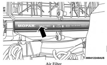
6. Install the A/C air filter with the air filter position indicators pointing in the same direction as removal.
