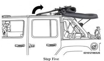
NOTE: If leaving the soft top in the Sunrider position, secure the top by using the two velcro straps provided in the center console.
