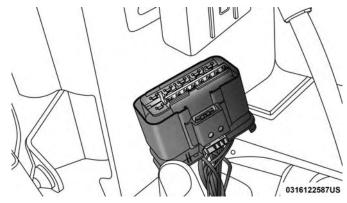
Pull Wiring Harness To Separate
