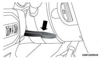
Tilt/Telescoping Steering Column Lever
