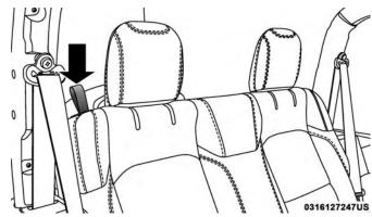
Rear Head Restraint Folding Strap Location
