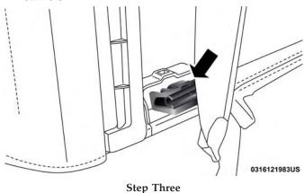
4. Line up the rear window to the **passenger side** quarter window first, and engage the plastic retainers.
