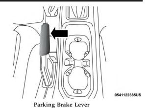
When the parking brake is applied with the ignition switch ON, the "Brake Warning Light" in the instrument cluster will illuminate.
