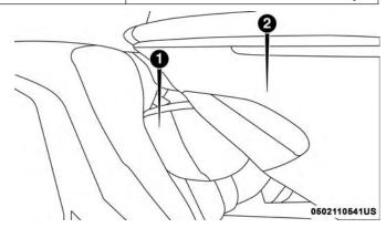
Car Seat With Head Restraint Folded
