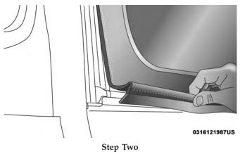
3. Remove plastic retainer from the bottom to the top of the front window.
