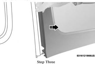
4. While keeping the window level, slide rearward until it is completely separate from its retainer. Do not pull downward while removing the window. Damage to the retainer could result.
