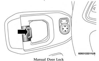
**NOTE:** The mechanical flip key can be used to lock or unlock the doors, swing gate, glove compartment, and console storage.
