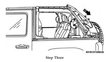
4. While pushing downward slightly on the folded soft top, slide the lock lever on the driver and passenger side lift assist mechanisms to the "lock" position.
