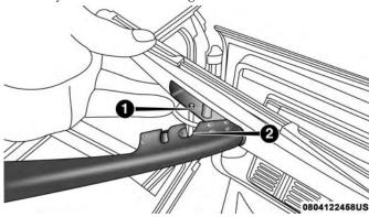
Wiper Blade Removed From Wiper Arm
