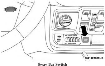
Push the SWAY BAR switch to activate the system. Push the switch again to deactivate the system. The "Sway Bar Indicator Light" (located in the instrument cluster) will illuminate when the bar is disconnected. The "Sway Bar Indicator Light" will flash during activation transition, or when activation conditions are not met. The stabilizer/sway bar should remain in on-road mode during normal driving conditions.
