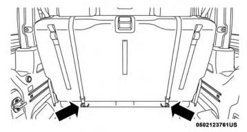
Tether Strap Anchorages (Two-Door Models) Four-Door Models:
