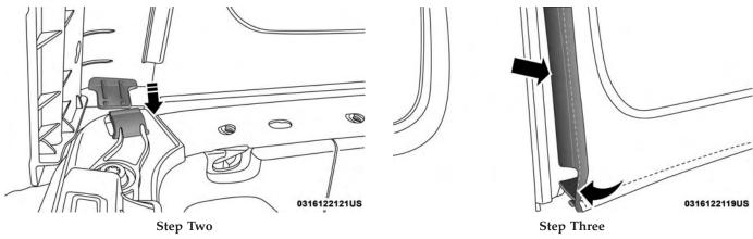
3. Engage the plastic retainers along the bottom of the quarter window and up the front of the window. Repeat on the other side.
