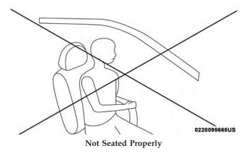
• If a child restraint system, child, small teenager or adult in the front passenger seat is seated improperly, the occupant may provide an output signal to the OCS that is different from the occupant's properly seated weight input. This may result in serious injury or death in a collision.
