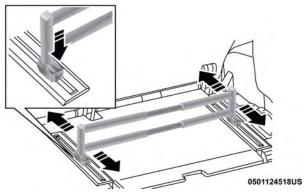
Lower Bar Into Slides — Slide To Adjust
