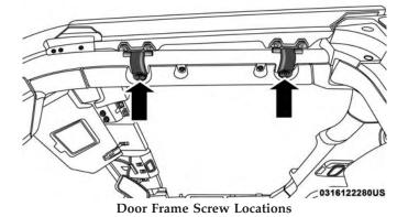
2. Once all the way loosened, remove the screws by pulling downward.
